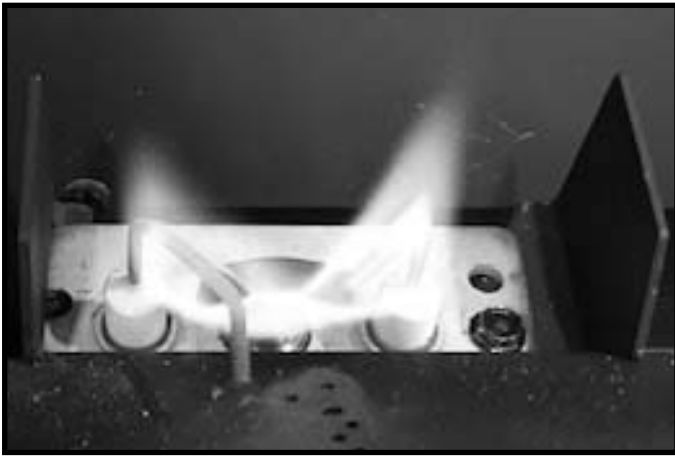
Figure 4.2 IPI Pilot Flame Patterns
