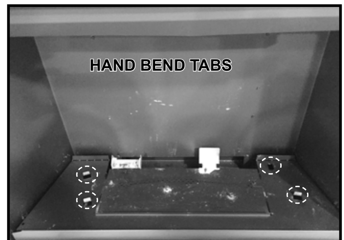
Figure 3. Hand Bend Tab Locations - QUARTZ36 Shown
