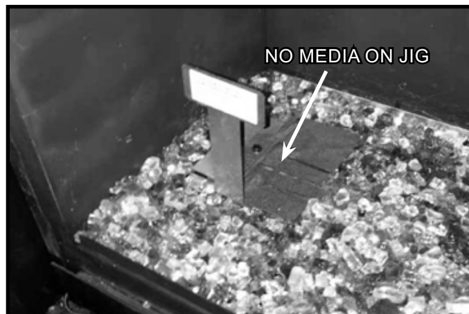
Figure 2. Media Placement Jig in Place
